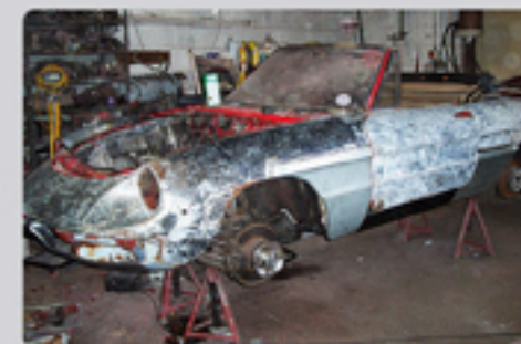
The Spider had its front valance cut out and work began to replace the rotten front crossmember – a very involved job.
